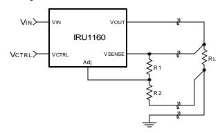
Figure 4 - Schematic showing connection for best load regulation.
