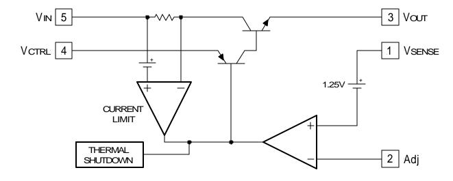
Figure 2 - Simplified block diagram of the IRU1160.
