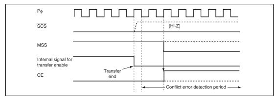
Figure 14.11 Conflict Error Detection Timing (After Transfer End)
