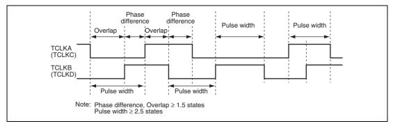
Figure 10.46 Phase Difference, Overlap, and Pulse Width in Phase Counting Mode
