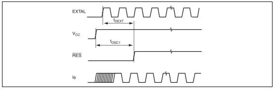
Figure 21.4 Oscillation Settling Timing
