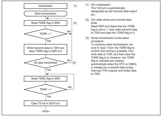
Figure 13.17 Sample Serial Transmission Flowchart
