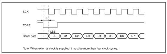
Figure 13.33 Sample Transmission using DTC or DMAC in Clocked Synchronous Mode
