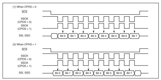
Figure 14.2 Relationship of Clock Phase, Polarity, and Data
