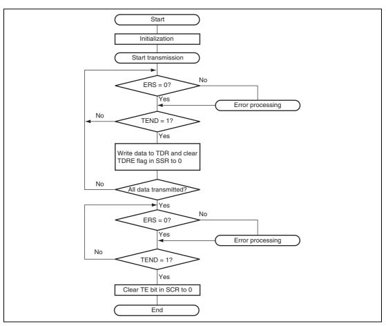
Figure 13.28 Sample Transmission Flowchart
