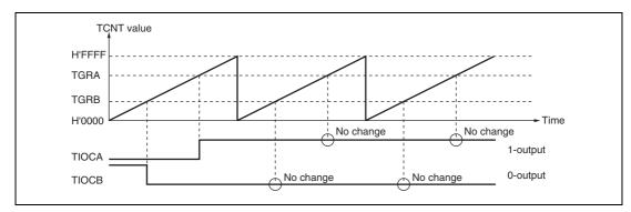
Figure 10.7 Example of 0-Output/1-Output Operation
