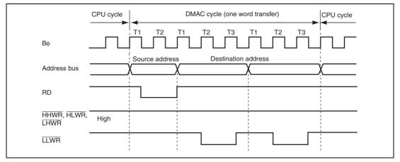
Figure 7.23 Example of Bus Timing of DMA Transfer
