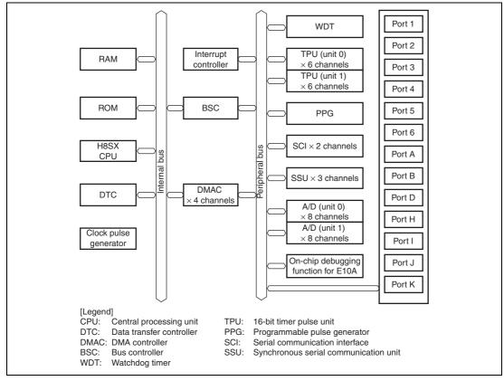
Figure 1.1 Block Diagram of H8SX/1582
