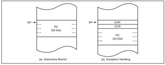
Figure 2.7 Stack Structure (Maximum Mode)
