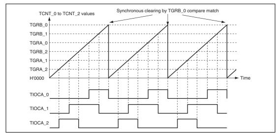
Figure 10.12 Example of Synchronous Operation
