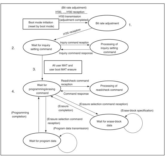
Figure 17.8 Boot Mode State Transition Diagram
