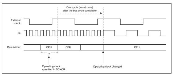
Figure 18.5 Clock Modification Timing
