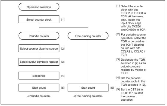
Figure 10.3 Example of Counter Operation Setting Procedure
