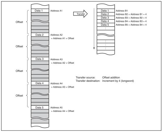
Figure 7.18 Operation of Offset Addition
