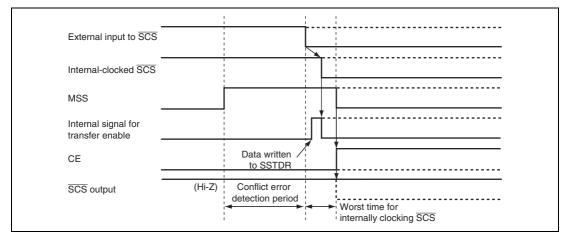
Figure 14.10 Conflict Error Detection Timing (Before Transfer)
