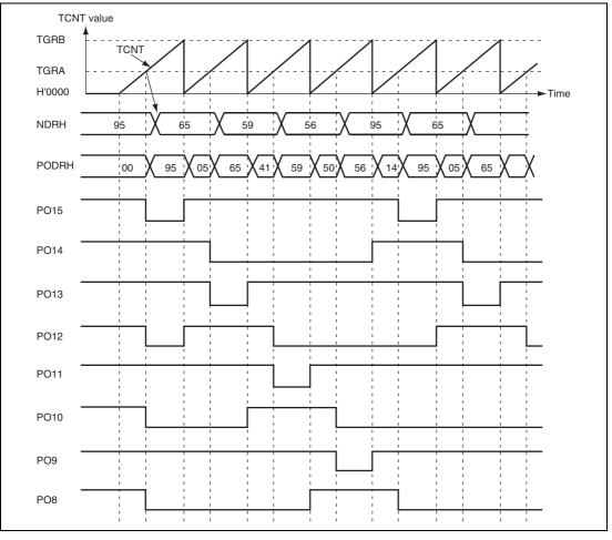
Figure 11.10 Inverted Pulse Output (Example)
