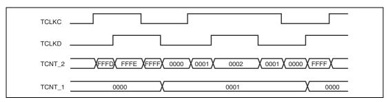
Figure 10.20 Example of Cascaded Operation (2)
