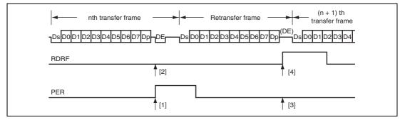
Figure 13.29 Data Re-Transfer Operation in SCI Reception Mode
