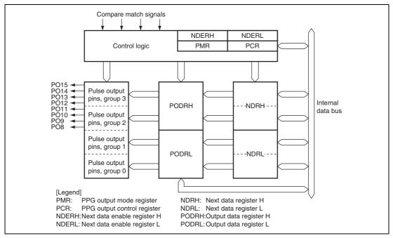
Figure 11.1 Block Diagram of PPG
