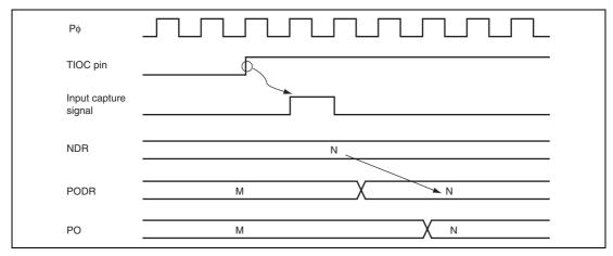
Figure 11.11 Pulse Output Triggered by Input Capture (Example)
