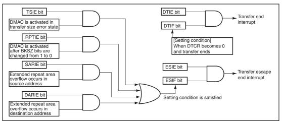
Figure 7.38 Interrupt and Interrupt Sources
