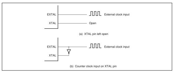
Figure 18.4 External Clock Input (Examples)
