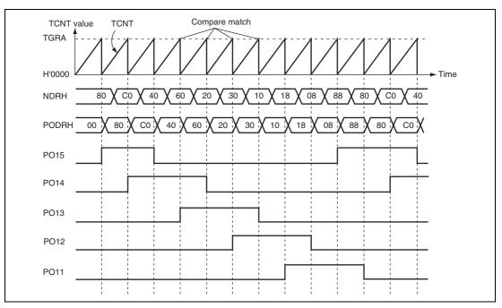
Figure 11.5 Normal Pulse Output Example (5-Phase Pulse Output)
