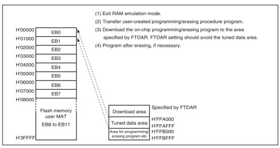
Figure 17.19 Programming Tuned Data
