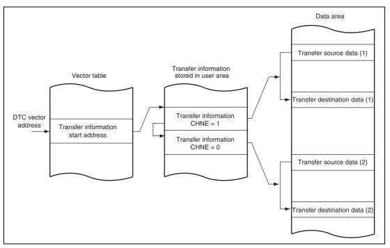
Figure 8.10 Operation of Chain Transfer
