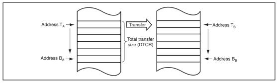
Figure 7.8 Operations in Normal Transfer Mode
