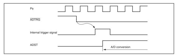
Figure 15.6 External Trigger Input Timing
