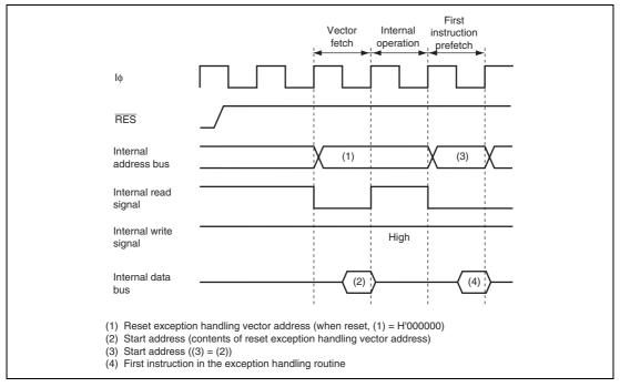
Figure 4.1 Reset Sequence (On-Chip ROM Enabled Advanced Mode)
