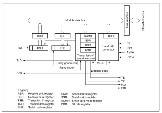
Figure 13.1 Block Diagram of SCI
