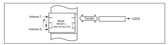
Figure 7.11 Operation in Single Address Mode in Block Transfer Mode (Block Area Specified)
