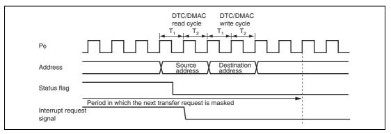
Figure 10.44 Timing for Status Flag Clearing by DMAC Activation (1)
