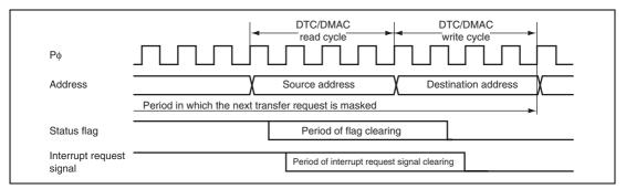
Figure 10.45 Timing for Status Flag Clearing by DMAC Activation (2)
