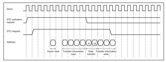
Figure 8.14 DTC Operation Timing (Example of Full Address Mode in Normal Transfer Mode or Repeat Transfer Mode)
