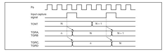
Figure 10.38 Buffer Operation Timing (Input Capture)
