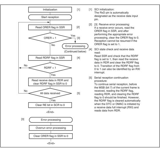
Figure 13.19 Sample Serial Reception Flowchart
