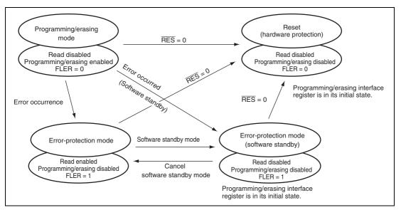
Figure 17.16 Transitions to Error Protection State
