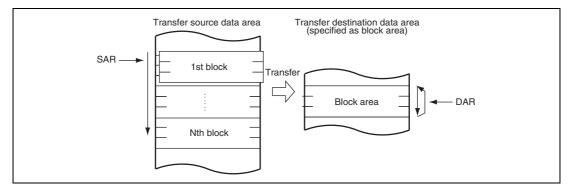
Figure 8.9 Memory Map in Block Transfer Mode (When Transfer Destination is Specified as Block Area)
