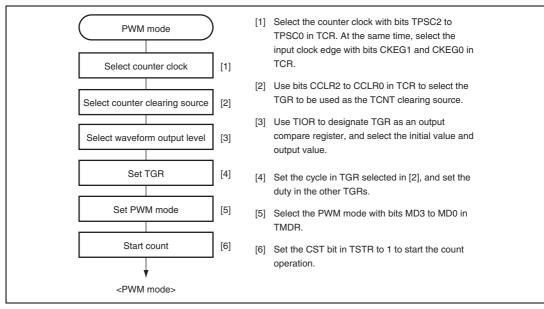
Figure 10.21 Example of PWM Mode Setting Procedure
