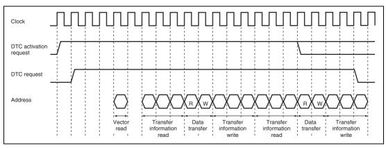
Figure 8.13 DTC Operation Timing (Example of Short Address Mode in Chain Transfer)
