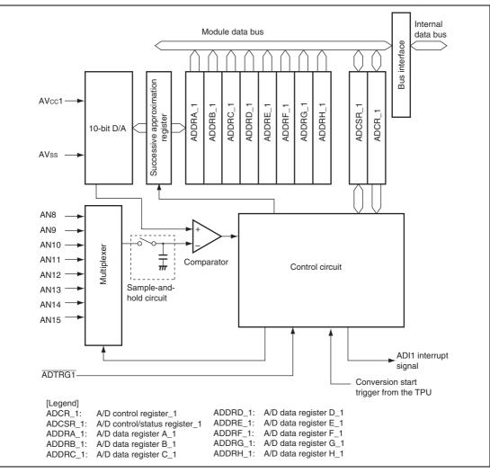
Figure 15.2 Block Diagram of A/D Converter (Unit 1/AD\_1)
