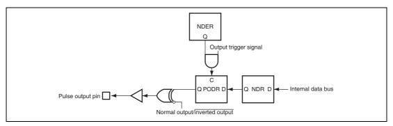
Figure 11.2 Schematic Diagram of PPG
