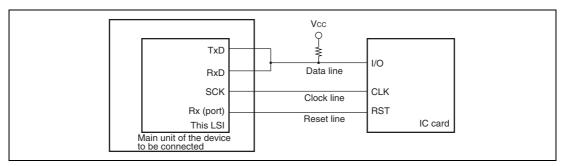
Figure 13.21 Pin Connection for Smart Card Interface
