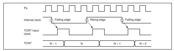
Figure 10.31 Count Timing in Internal Clock Operation
