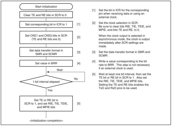
Figure 13.5 Sample SCI Initialization Flowchart
