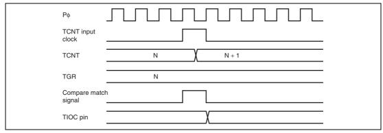
Figure 10.33 Output Compare Output Timing
