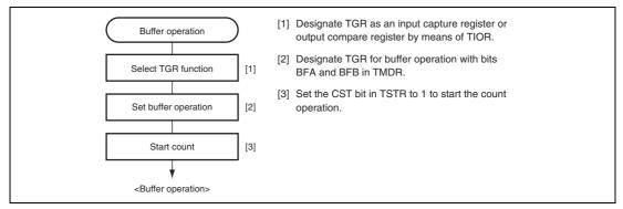
Figure 10.15 Example of Buffer Operation Setting Procedure
