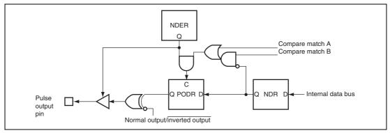
Figure 11.6 Non-Overlapping Pulse Output
