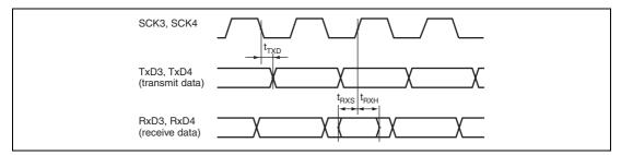
Figure 21.14 SCI Input/Output Timing: Clocked Synchronous Mode
