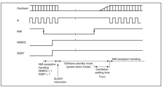
Figure 21.3 Oscillation Settling Timing after Software Standby Mode
