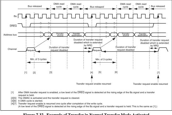
Figure 7.32 Example of Transfer in Normal Transfer Mode Activated by DREQ Low Level with NRD = 1
