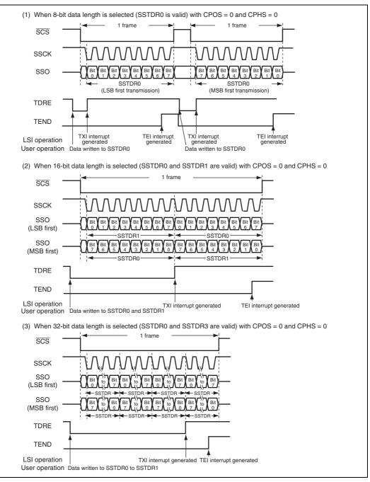
Figure 14.5 Example of Transmission Operation (SSU Mode)
