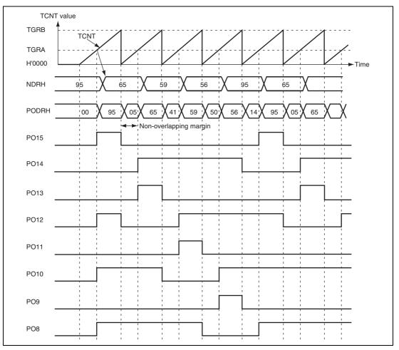
Figure 11.9 Non-Overlapping Pulse Output Example (4-Phase Complementary)
