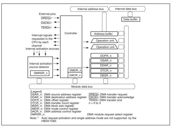
A block diagram of the DMAC is shown in figure 7.1.
