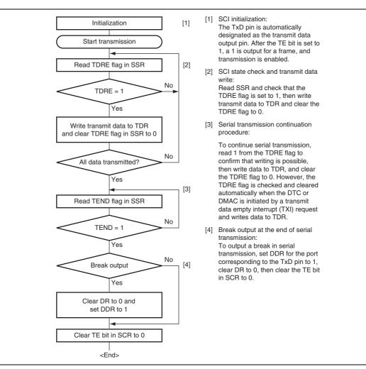
Figure 13.7 Sample Serial Transmission Flowchart
