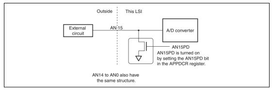
Figure 15.9 Diagram of Analog Port Pull-Down Function
