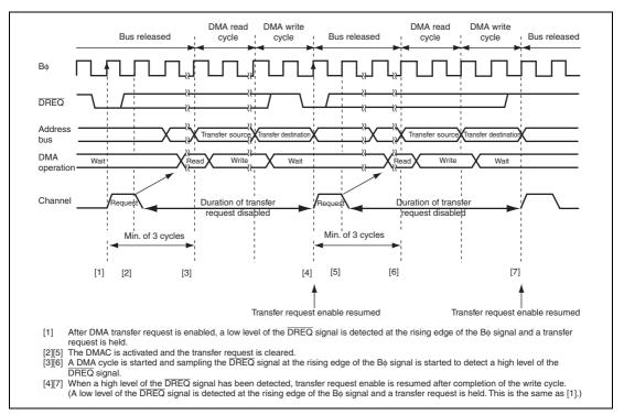
Figure 7.29 Example of Transfer in Normal Transfer Mode Activated by DREQ Falling Edge
