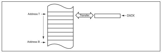
Figure 7.6 Operations in Single Address Mode
