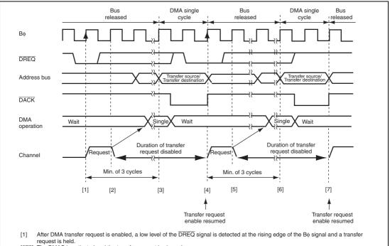
[2][5] The DMAC is activated and the transfer request is cleared.
