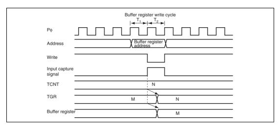
Figure 10.53 Conflict between Buffer Register Write and Input Capture
