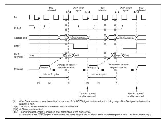
Figure 7.36 Example of Transfer in Single Address Mode Activated by DREQ Low Level
