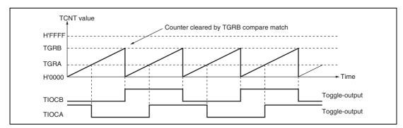
Figure 10.8 Example of Toggle Output Operation
