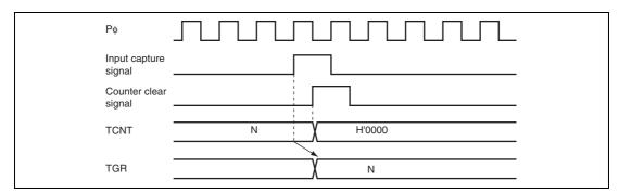
Figure 10.36 Counter Clear Timing (Input Capture)
