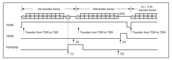
Figure 13.26 Data Re-Transfer Operation in SCI Transmission Mode
