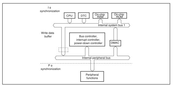
Figure 6.2 Internal Bus Configuration
