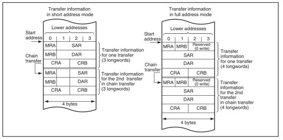
Figure 8.2 Transfer Information on Data Area
