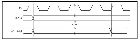
Figure 21.9 Data Input Timing for Realtime Input Port
