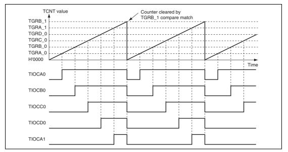
Figure 10.23 Example of PWM Mode Operation (2)
