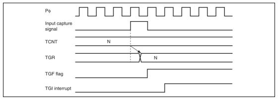
Figure 10.40 TGI Interrupt Timing (Input Capture)
