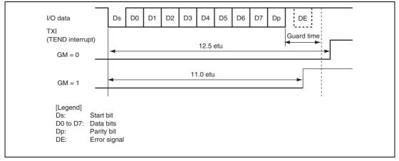
Figure 13.27 TEND Flag Set Timing during Transmission
