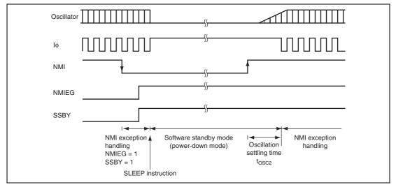
Figure 19.2 Software Standby Mode Application Example
