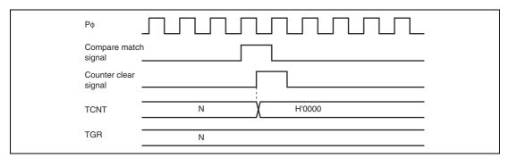
Figure 10.35 Counter Clear Timing (Compare Match)
