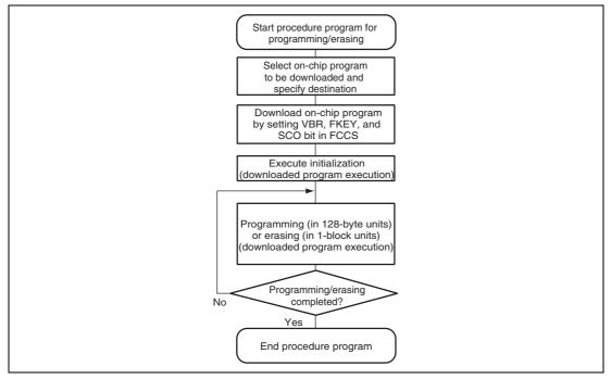
Figure 17.5 Procedure for Creating Procedure Program
