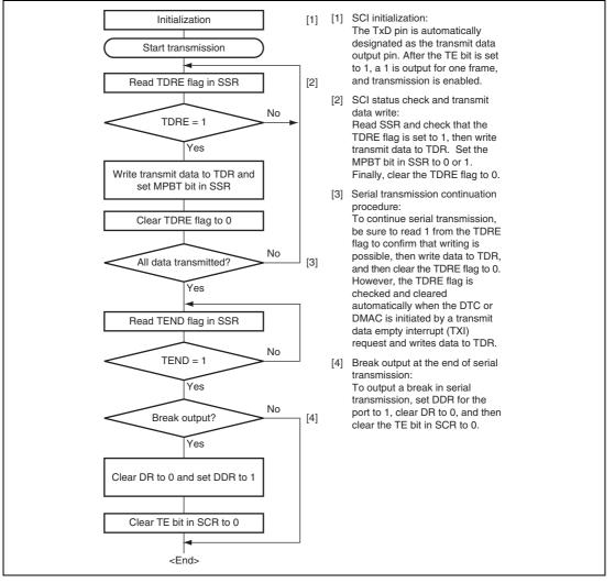
Figure 13.11 Sample Multiprocessor Serial Transmission Flowchart
