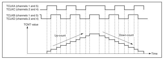
Figure 10.26 Example of Phase Counting Mode 1 Operation
