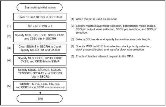
Figure 14.4 Example of Initial Settings in SSU Mode
