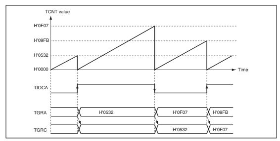
Figure 10.17 Example of Buffer Operation (2)
