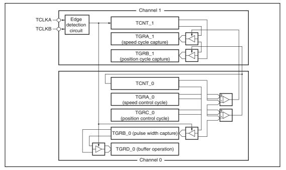
Figure 10.30 Phase Counting Mode Application Example
