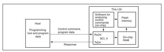
Figure 17.6 System Configuration in Boot Mode
