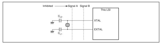
Figure 18.6 Note on Board Design for Oscillation Circuit
