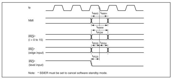
Figure 21.7 Interrupt Input Timing
