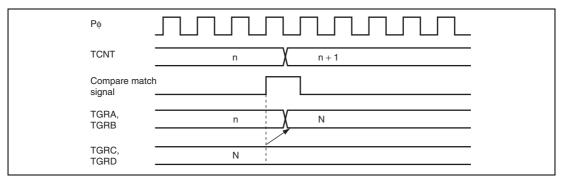
Figures 10.37 and 10.38 show the timings in buffer operation.
