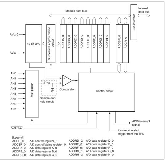
Figure 15.1 Block Diagram of A/D Converter (Unit 0/AD\_0)
