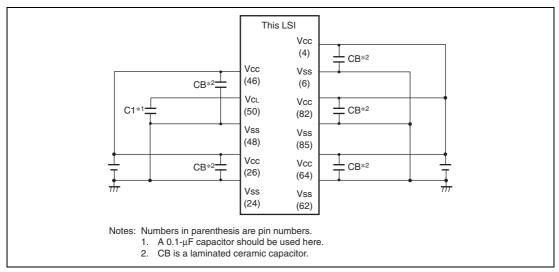
Figure 18.7 Connection Example of Bypass Capacitor
