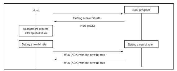
Figure 17.24 New Bit-Rate Selection Sequence
