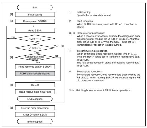
Figure 14.8 Flowchart Example of Data Reception (SSU Mode)
