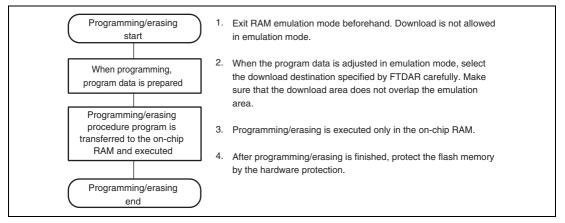
Figure 17.9 Programming/Erasing Flow
