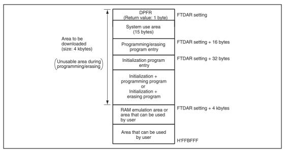
Figure 17.10 RAM Map when Programming/Erasing is Executed
