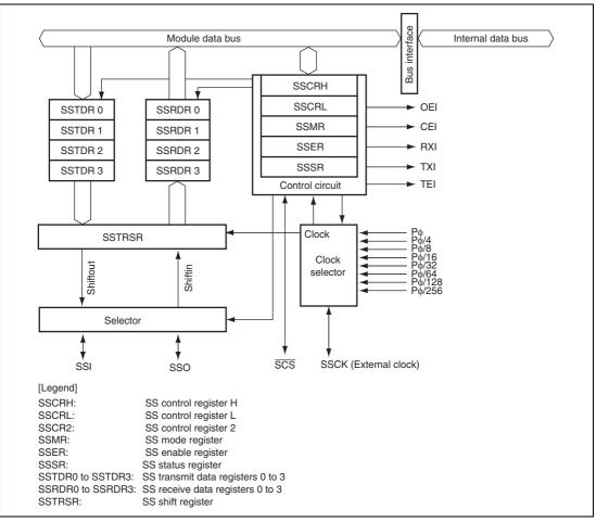
Figure 14.1 Block Diagram of SSU
