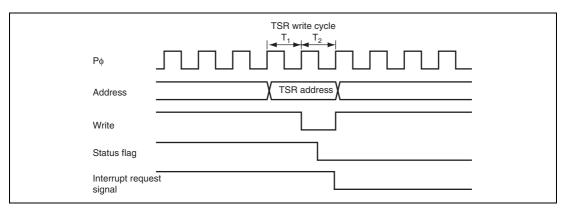
Figure 10.43 Timing for Status Flag Clearing by CPU
