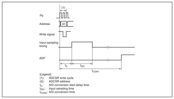
Figure 15.5 A/D Conversion Timing
