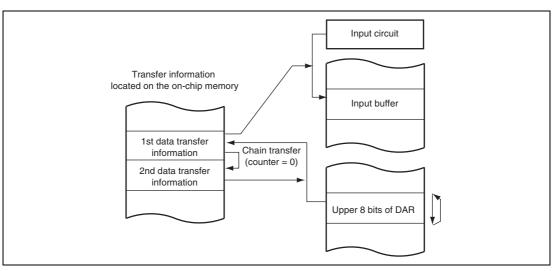
Figure 8.16 Chain Transfer when Counter = 0
