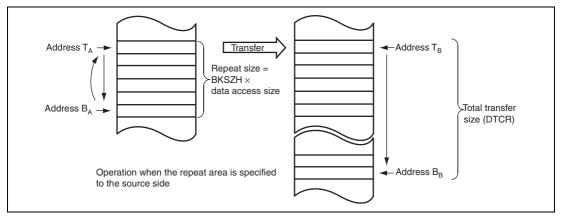
Figure 7.9 Operations in Repeat Transfer Mode
