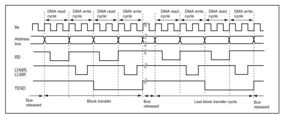
Figure 7.28 Example of Transfer in Block Transfer Mode
