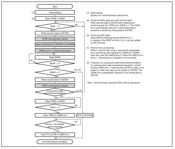
Figure 14.9 Flowchart Example of Simultaneous Transmission/Reception (SSU Mode)
