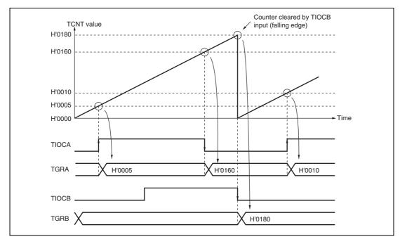
Figure 10.10 Example of Input Capture Operation
