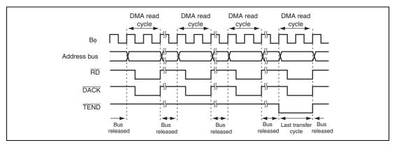
Figure 7.33 Example of Transfer in Single Address Mode (Byte Read)
