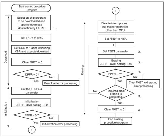
Figure 17.12 Erasing Procedure in User Program Mode
