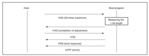
Figure 17.22 Bit-Rate-Adjustment Sequence
