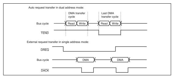
Figure 7.7 Example of Signal Timing in Normal Transfer Mode
