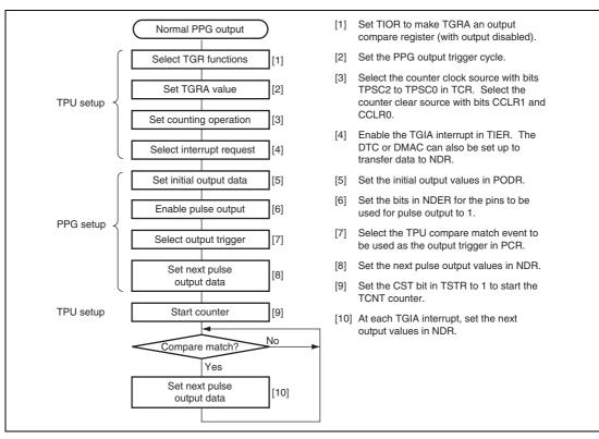
Figure 11.4 Setup Procedure for Normal Pulse Output (Example)
