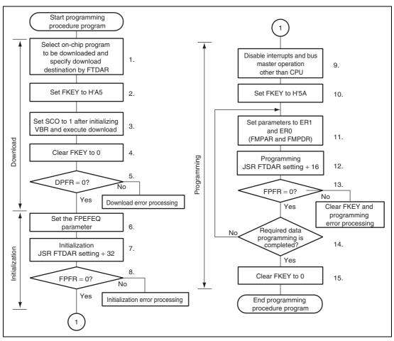
Figure 17.11 Programming Procedure in User Program Mode
