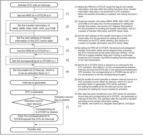
Figure 8.15 Using DTC with Interrupt Activation
