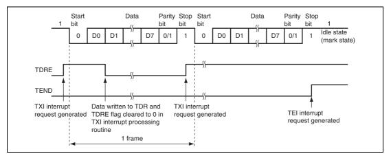
Figure 13.6 Example of Operation for Transmission in Asynchronous Mode (Example with 8-Bit Data, Parity, One Stop Bit)
