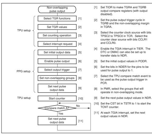
Figure 11.8 Setup Procedure for Non-Overlapping Pulse Output (Example)
