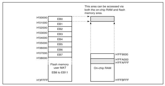
Figure 17.18 shows an example of overlaying flash memory block area EB0.
