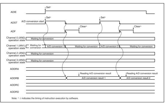
Figure 15.3 Example of A/D Converter Operation (Single Mode, Channel 1 Selected)
