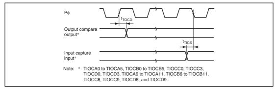
Figure 21.10 TPU Input/Output Timing
