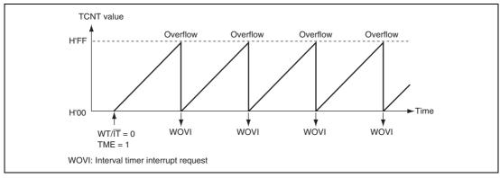
Figure 12.3 Operation in Interval Timer Mode
