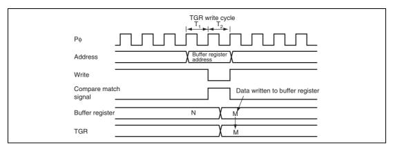
Figure 10.50 Conflict between Buffer Register Write and Compare Match
