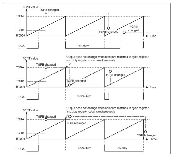
Figure 10.24 shows examples of PWM waveform output with 0% duty cycle and 100% duty cycle in PWM mode.
