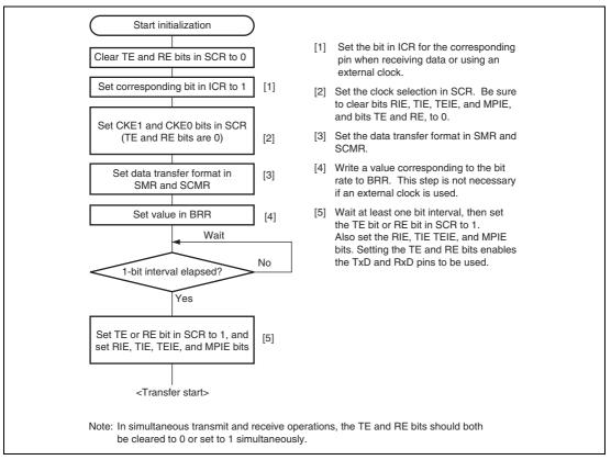
Figure 13.15 Sample SCI Initialization Flowchart
