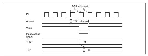
Figure 10.52 Conflict between TGR Write and Input Capture
