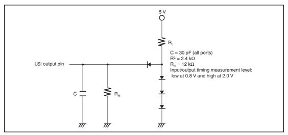
Figure 21.1 Output Load Circuit
