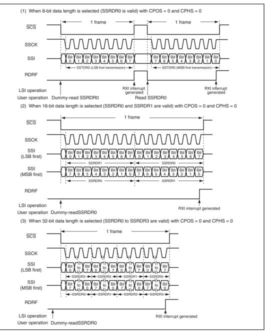
Figure 14.7 Example of Reception Operation (SSU Mode)
