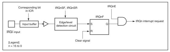
Figure 5.2 Block Diagram of Interrupts IRQn
