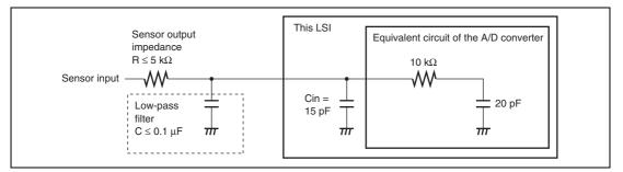
Figure 15.10 Example of Analog Input Circuit
