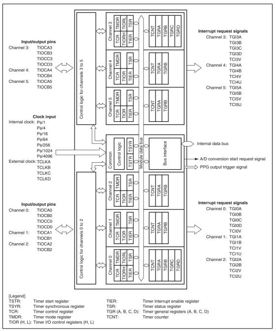
Figure 10.1 Block Diagram of TPU (Unit 0)
