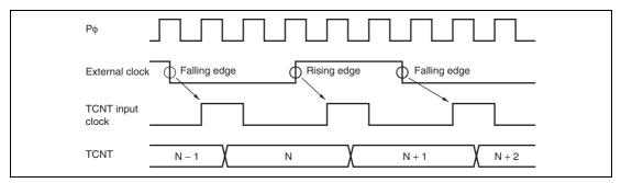
Figure 10.32 Count Timing in External Clock Operation
