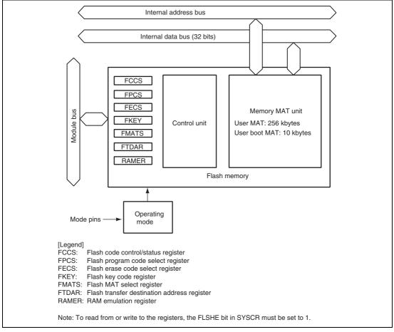
Figure 17.1 Block Diagram of Flash Memory
