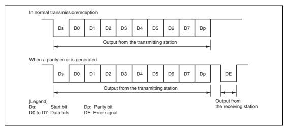
Figure 13.22 Data Formats in Normal Smart Card Interface Mode
