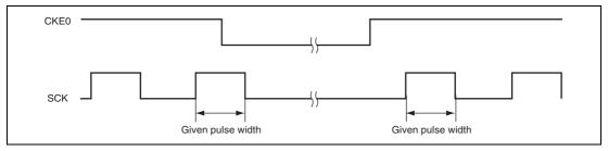
Figure 13.31 Clock Output Fixing Timing
