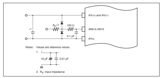
Figure 15.11 Example of Analog Input Protection Circuit
