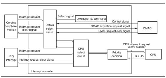
Figure 5.6 Block Diagram of DMAC and Interrupt Controller
