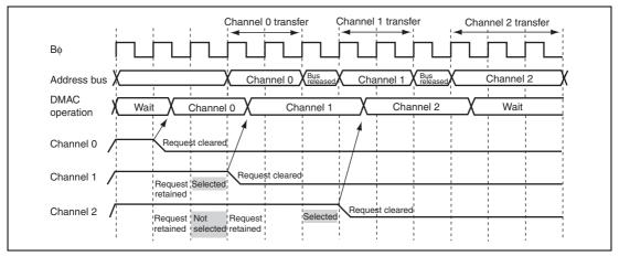
Figure 7.22 shows a transfer example when multiple transfer requests from channels 0 to 2.
