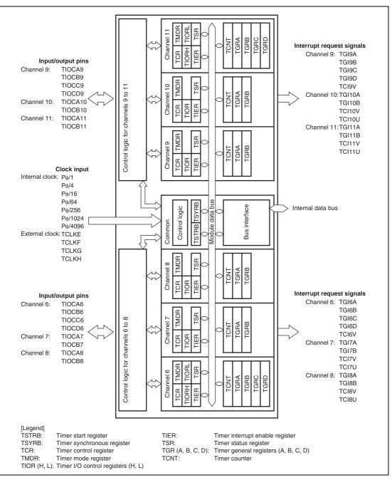
Figure 10.2 Block Diagram of TPU (Unit 1)
