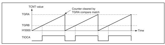
Figure 10.22 Example of PWM Mode Operation (1)
