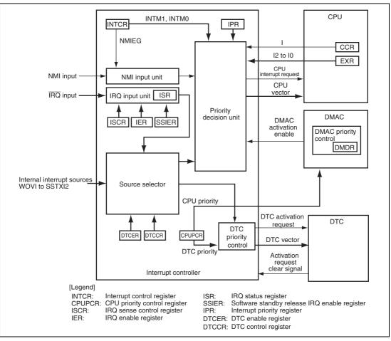
A block diagram of the interrupt controller is shown in figure 5.1.
