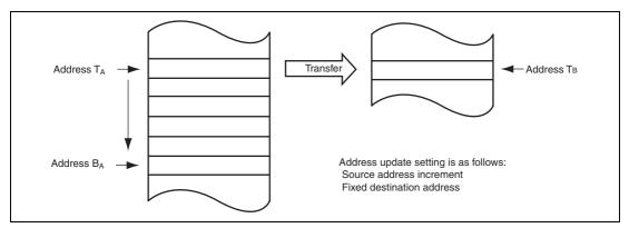
Figure 7.3 Operations in Dual Address Mode
