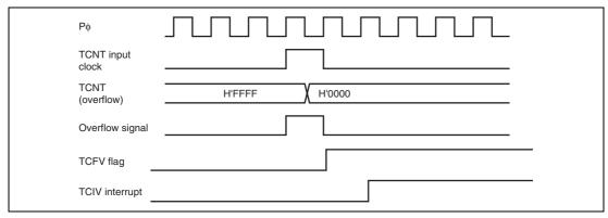
Figure 10.41 TCIV Interrupt Setting Timing
