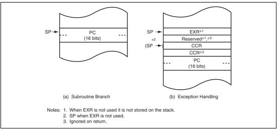
Figure 2.3 Stack Structure (Normal Mode)
