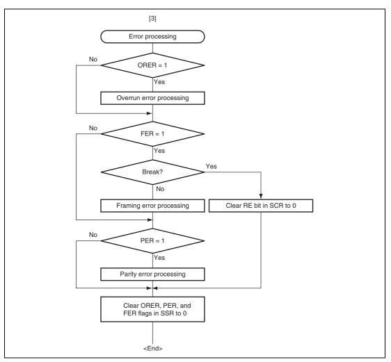
Figure 13.9 Sample Serial Reception Flowchart (2)
