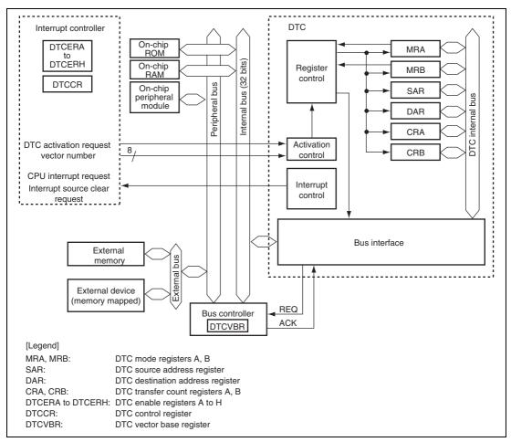
Figure 8.1 Block Diagram of DTC
