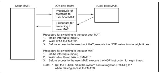
Figure 17.20 Switching between User MAT and User Boot MAT
