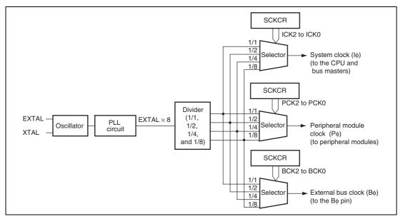
Figure 18.1 Block Diagram of Clock Pulse Generator
