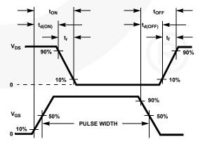
Figure 20. Switching Time Waveforms
