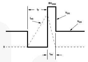
Figure 16. Unclamped Energy Waveforms
