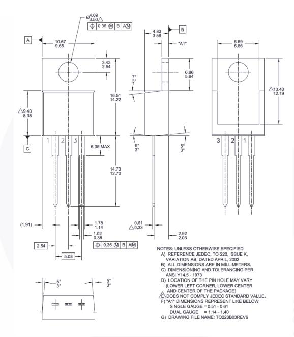
Figure 22. TO-220, Molded, 3Lead, Jedec Variation AB
