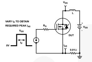
Figure 15. Unclamped Energy Test Circuit
