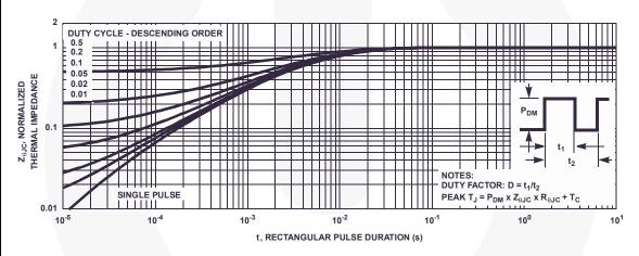
Figure 3. Normalized Maximum Transient Thermal Impedance
