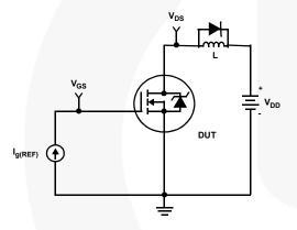
Figure 17. Gate Charge Test Circuit
