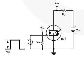
Figure 19. Switching Time Test Circuit
