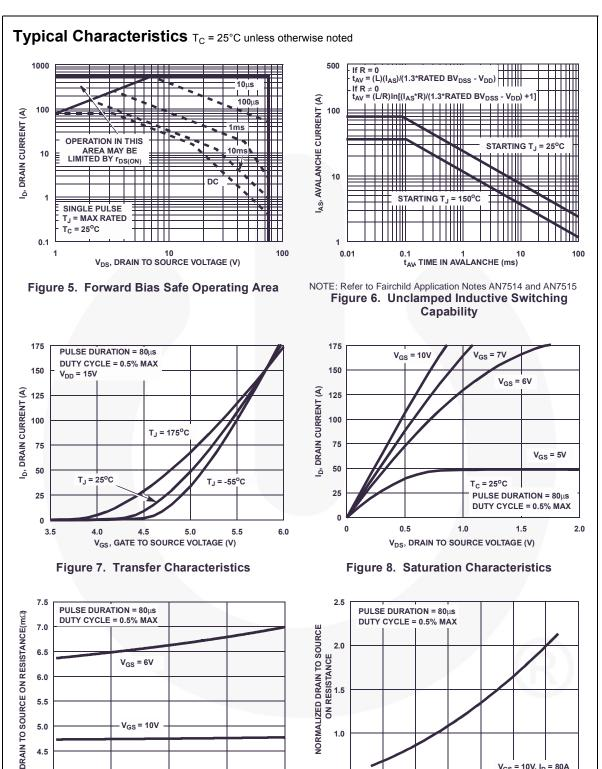
Figure 9. Drain to Source On Resistance vs Drain Current
