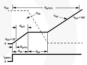
Figure 18. Gate Charge Waveforms
