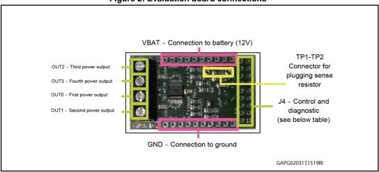
Figure 2: Evaluation board connections
