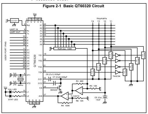
If there is a large amount of coupling between X and Y lines, and where burst length 'n' is set to a high number, charge accumulation on Cs may reach a point where the ladder DAC can no longer offset the signal back into the ADC's usable range. In this case the circuit will employ one or two of the Cz capacitors to 'knock back' or cancel the charge accumulated
