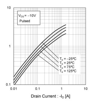
Gate Threshold Voltage: -V<sub>GS(th)</sub> [V]
