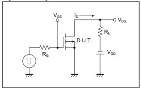
Fig.2-1 Gate Charge Measurement Circuit
