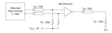
Figure 6. PCLK MPC9456 AC test reference for  $V_{CC}$  = 3.3V and  $V_{CC}$  = 2.5V
