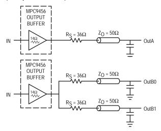
Figure 3. Single versus Dual Transmission Lines
