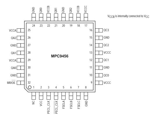
Figure 2. Pinout: 32–Lead Package Pinout (Top View)
