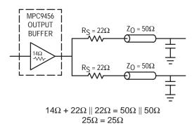
Figure 5. Optimized Dual Line Termination
