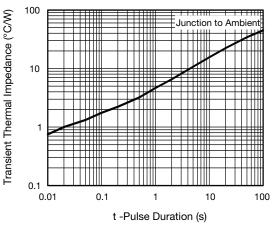
Fig. 6 - Typical Transient Thermal Impedance Per Device
