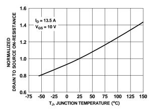
Figure 3. Normalized On-Resistance vs Junction Temperature
