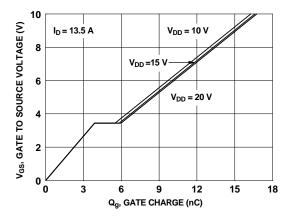
Figure 7. Gate Charge Characteristics
