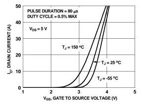
Figure 5. Transfer Characteristics
