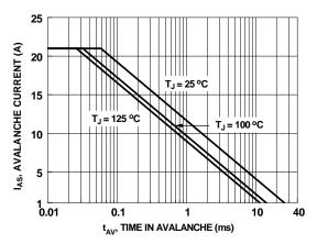
Figure 9. Unclamped Inductive Switching Capability
