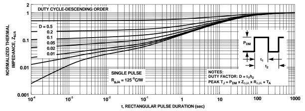
Figure 13. Junction-to-Ambient Transient Thermal Response Curve
