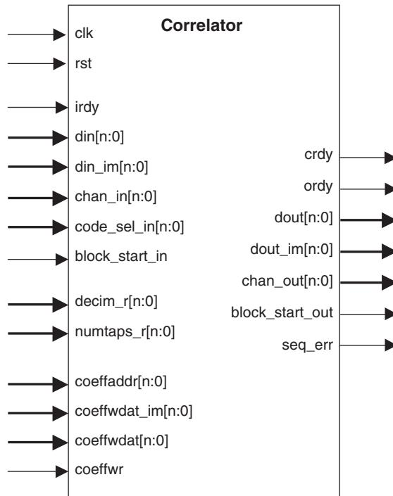
The Correlator IP core circuit is shown in the following block diagram.
