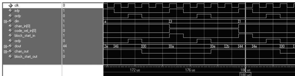
**Figure 4. User Interface Timing Diagram for Two-channel Correlator**
