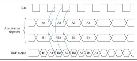
The Arria GX IOE operates in bidirectional DDR mode by combining the DDR input and DDR output configurations. The negative-edge-clocked OE register holds the OE signal inactive until the falling edge of the clock to meet DDR SDRAM timing requirements.
