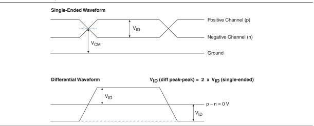
Figure 4-4. Transmitter Output Waveform
