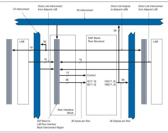
Figure 2–53. DSP Block Interface to Interconnect
