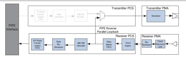
You can dynamically put the PCI Express (PIPE) mode transceiver in reverse parallel loopback by controlling the tx\_detectrxloopback port instantiated in the MegaWizard Plug-In Manager. A high on the tx\_detectrxloopback port in P0 power state puts the transceiver in reverse parallel loopback. A high on the tx\_detectrxloopback port in any other power state does not put the transceiver in reverse parallel loopback.
