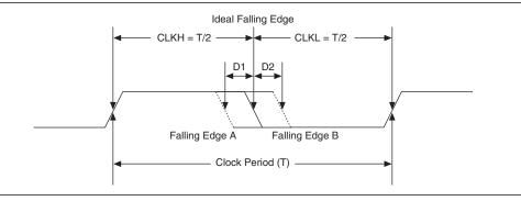
DCD expressed in absolution derivation, for example, D1 or D2 in Figure 4–10, is clock-period independent. DCD can also be expressed as a percentage, and the percentage number is clock-period dependent. DCD as a percentage is defined as:
