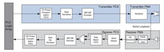
In GIGE and Serial RapidIO modes, you can dynamically put each transceiver channel individually in serial loopback by controlling the rx\_seriallpbken port. A high on the rx\_seriallpbken port puts the transceiver into serial loopback and a low takes the transceiver out of serial loopback.
