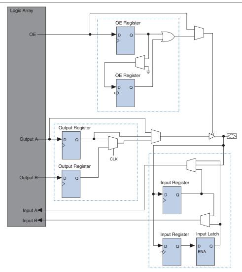
The IOEs are located in I/O blocks around the periphery of the Arria GX device. There are up to four IOEs per row I/O block and four IOEs per column I/O block. Row I/O blocks drive row, column, or direct link interconnects. Column I/O blocks drive column interconnects.
