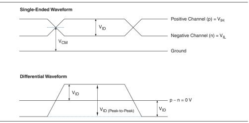
Figure 4–6. Transmitter Output Waveforms for Differential I/O Standards
