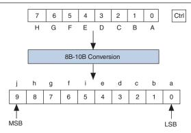
During reset (tx\_digitalreset), the running disparity and data registers are cleared and the 8B/10B encoder continously outputs a K28.5 pattern from the RD-column. After out of reset, the 8B/10B encoder starts with a negative disparity (RD-) and transmits three K28.5 code groups for synchronizing before it starts encoding the input data or control character.
