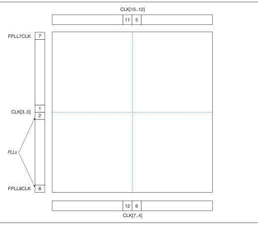
Figure 2–62 and Figure 2–63 shows global and regional clocking from the fast PLL outputs and side clock pins. The connections to the global and regional clocks from the fast PLL outputs, internal drivers, and CLK pins on the left side of the device are shown in Table 2–19.
