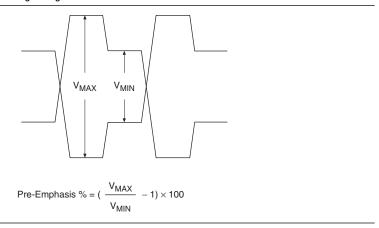
Pre-emphasis percentage is defined as  $(V_{MAX}/V_{MIN}-1)\times 100$ , where  $V_{MAX}$  is the differential emphasized voltage (peak-to-peak) and  $V_{MIN}$  is the differential steady-state voltage (peak-to-peak).
