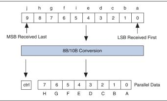
If the received 10-bit code is not a part of valid Dx.y or Kx.y code groups, the 8B/10B decoder block asserts an error flag on the rx\_errdetect port. If the received 10-bit code is detected with incorrect running disparity, the 8B/10B decoder block asserts an error flag on the rx\_disperr and rx\_errdetect ports. The error flag signals (rx\_errdetect and rx\_disperr) have the same data path delay from the 8B/10B decoder to the PLD-transceiver interface as the bad code group.
