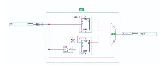
When an FPGA PLL generates the internal clock, the PLL output clocks the IOE block. As the PLL only monitors the positive edge of the reference clock input and internally re-creates the output clock signal, any DCD present on the reference clock is filtered out. Therefore, the DCD for a DDIO output with PLL in the clock path is better than the DCD for a DDIO output without PLL in the clock path.
