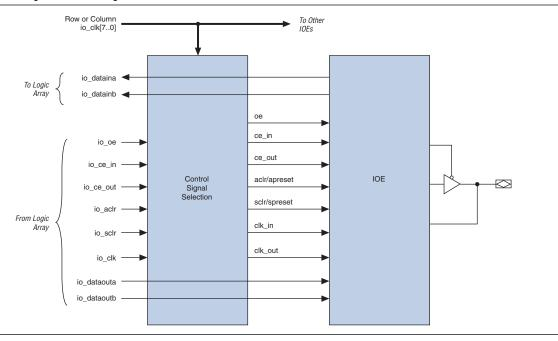
Each IOE contains its own control signal selection for the following control signals: oe, ce\_in, ce\_out, aclr/apreset, sclr/spreset, clk\_in, and clk\_out. Figure 2–71 shows the control signal selection.
