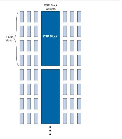
Table 2–13 lists the number of DSP blocks in each Arria GX device. DSP block multipliers can optionally feed an adder/subtractor or accumulator in the block depending on the configuration, which makes routing to ALMs easier, saves ALM routing resources, and increases performance because all connections and blocks are in the DSP block.
