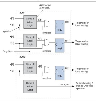
Figure 2–35. Conditional Operation Example
