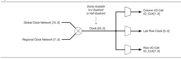
You can use the Quartus II software to control whether a clock input pin drives either a GCLK, RCLK, or dual-RCLK network. The Quartus II software automatically selects the clocking resources if not specified.
