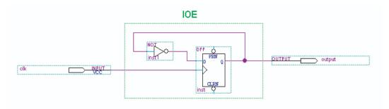
However, when the output is a double data rate input/output (DDIO) signal, both edges of the input clock signal (positive and negative) trigger output transitions (Figure 4–12). Therefore, any distortion on the input clock and the input clock buffer affect the output DCD.
