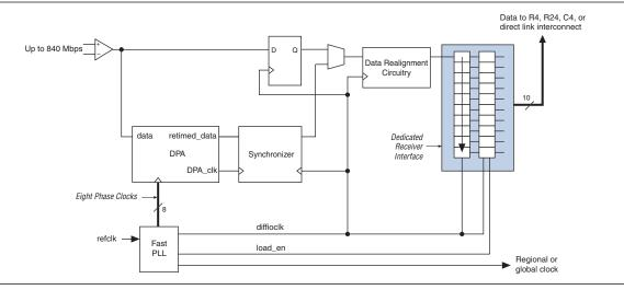
An external pin or global or regional clock can drive the fast PLLs, which can output up to three clocks: two multiplied high-speed clocks to drive the SERDES block and/or external pin, and a low-speed clock to drive the logic array. In addition, eight phase-shifted clocks from the  $V_{CO}$  can feed to the DPA circuitry.
