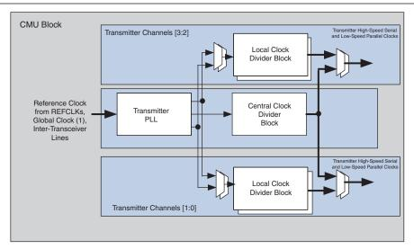
The transmitter PLL multiplies the input reference clock to generate the high-speed serial clock required to support the intended protocol. It implements a half-rate voltage controlled oscillator (VCO) that generates a clock at half the frequency of the serial data rate for which it is configured.
