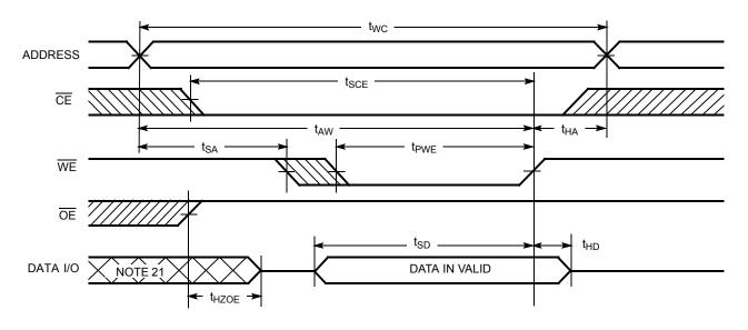
Figure 8. Write Cycle No. 3 (WE Controlled, OE LOW) [20]
