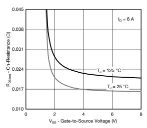
On-Resistance vs. Gate-to-Source Voltage
