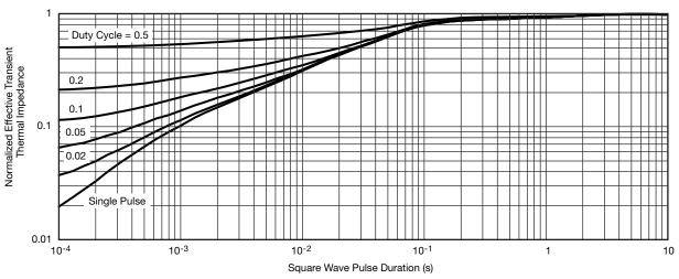
Normalized Thermal Transient Impedance, Junction-to-Foot
