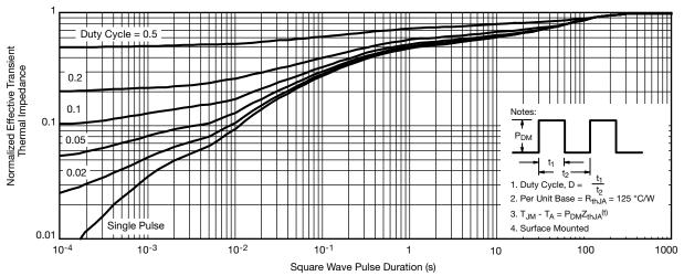
Normalized Thermal Transient Impedance, Junction-to-Ambient
