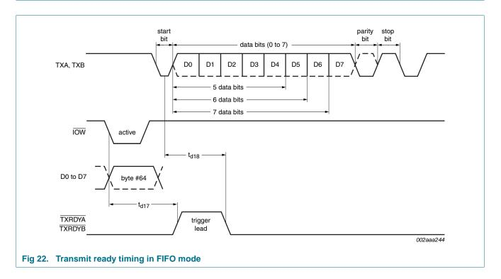
5 V, 2.2 V and 2.5 V dual UART, 5 Mbit/s (max.), with 64-byte FIFOs
