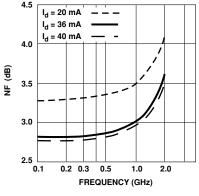
Figure 6. Noise Figure vs. Frequency.
