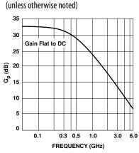
Figure 1. Typical Power Gain vs. Frequency,  $I_d = 36 \text{ mA}$ .
