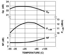
Figure 4. Output Power at 1 dB Gain Compression, NF and Power Gain vs. Case Temperature,  $f=1.0~{\rm GHz},$   $I_d=36~{\rm mA}.$
