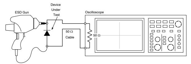
Figure 4. Diagram of ESD Test Setup
