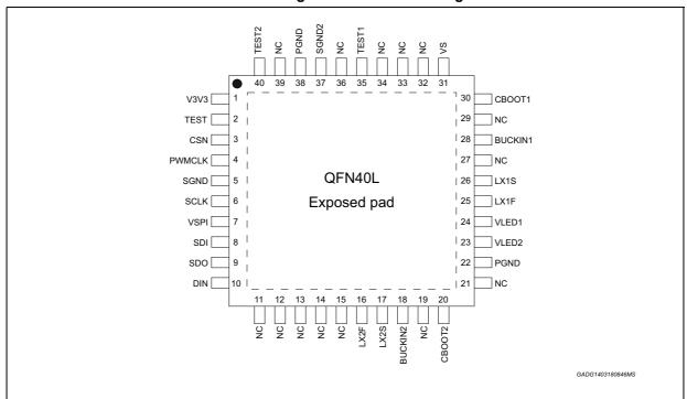
Figure 4. Connection diagram
