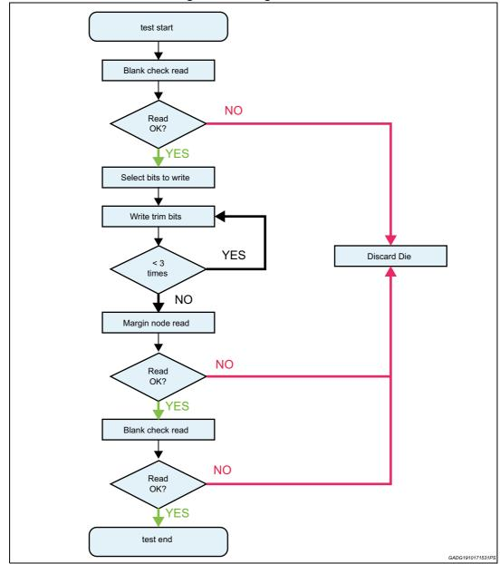
Figure 8. Testing flow chart
