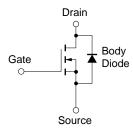
**Remark** Strong electric field, when exposed to this device, can cause destruction of the gate oxide and ultimately degrade the device operation. Steps must be taken to stop generation of static electricity as much as possible, and quickly dissipate it once, when it has occurred.
