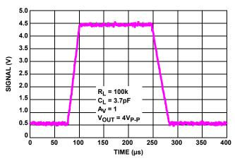
FIGURE 16. LARGE SIGNAL STEP RESPONSE (4V)
