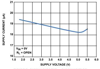
FIGURE 7. SUPPLY CURRENT vs SUPPLY VOLTAGE
