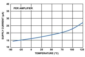
FIGURE 6. SUPPLY CURRENT vs TEMPERATURE,  $Vs = \pm 2.5V$
