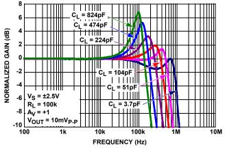
FIGURE 15. GAIN vs FREQUENCY vs CL
