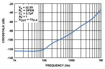
FIGURE 22. CROSSTALK vs FREQUENCY,  $V_S = \pm 2.5V$
