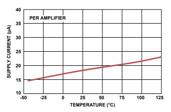
FIGURE 5. SUPPLY CURRENT vs TEMPERATURE,  $Vs = \pm 0.9V$
