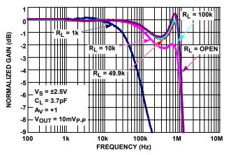
FIGURE 10. GAIN vs FREQUENCY vs  $R_L$ ,  $V_S = \pm 2.5V$
