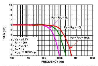
FIGURE 11. GAIN vs FREQUENCY vs FEEDBACK RESISTOR VALUES  $R_{\mbox{\scriptsize F}}/R_{\mbox{\scriptsize G}}$
