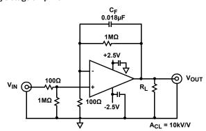
FIGURE 24. HIGH GAIN, PRECISION DC-COUPLED AMPLIFIER
