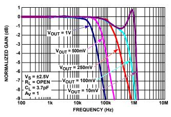
FIGURE 12. GAIN vs FREQUENCY vs Vout
