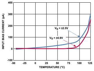
FIGURE 3. IB+ vs TEMPERATURE
