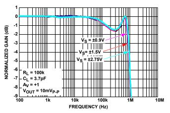
FIGURE 14. GAIN vs FREQUENCY vs SUPPLY VOLTAGE
