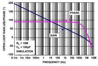
FIGURE 8. FREQUENCY RESPONSE vs OPEN LOOP GAIN,  $R_L = \text{10M}\Omega$
