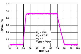
FIGURE 17. LARGE SIGNAL STEP RESPONSE (1V)
