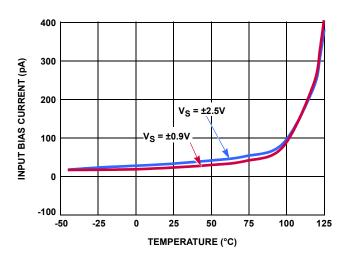
FIGURE 2. IB vs TEMPERATURE
