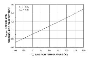
Figure 3. On-Resistance Variation withTemperature.
