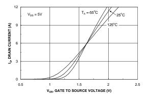
Figure 5. Transfer Characteristics.
