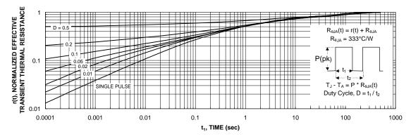
Figure 11. Transient Thermal Response Curve.
