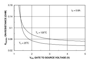
Figure 4. On-Resistance Variation with Gate-to-Source Voltage.
