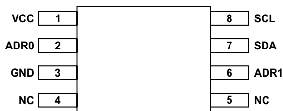
Package LE, 8-Pin TSSOP Pin-out Diagram
