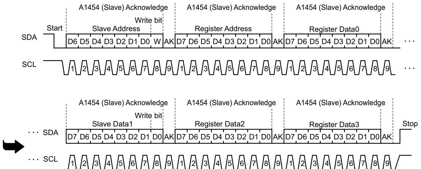
Figure 2: I 2 C Write Operation
