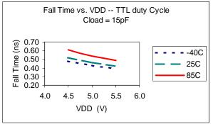
Figure 8. Rise/Fall Time vs. Output Loads over Temperatures
