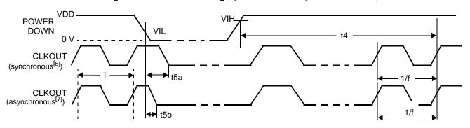
Figure 5. Power up Timing
