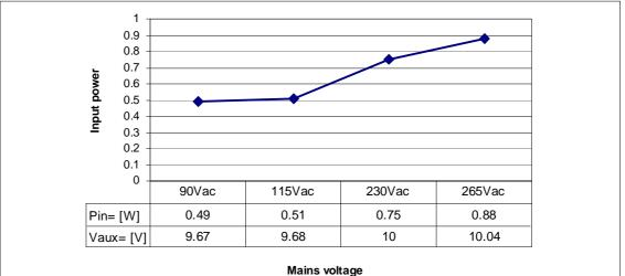
It is clearly visible that, while delivering the required standby load, (5V at 50mA, 1.8V, 3.3V and 12V at 0mA) *the input power consumption is below 800mW* at both the nominal input voltage ranges and remains below 900mW at 265Vac. *Figure 10.* represents the input power variation as a function of the 5V current.
