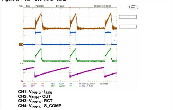
Figure 8. Vin = 230 Vrms - 50Hz
