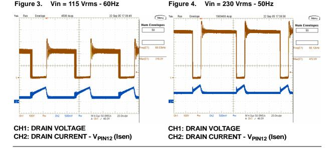
The pictures above show the drain voltage and current signal on pin #12 at the nominal input mains voltage during normal operation at full load. The Envelope acquisition of the scope provides for the possibility to observe the modulation of the two waveforms, due to the mains input voltage ripple at twice the line frequency.
