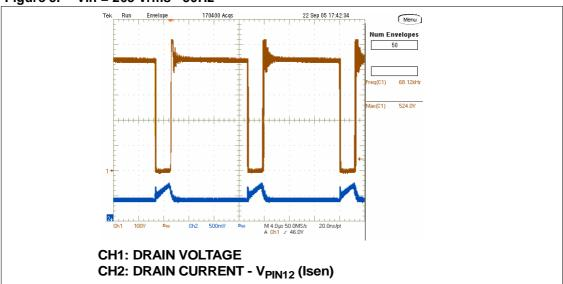
Figure 5. Vin = 265 Vrms - 50Hz
