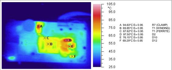
The thermistor, bridge and output diodes temperature rise are compatible with the reliable operation of the components. Resistor R7 may need a bigger package to decrease its thermal resistance. All other components of the board are working within the temperature limits assuring a reliable long term operation of the power supply.
