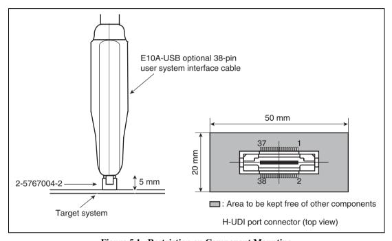
Figure 5.1 Restriction on Component Mounting
